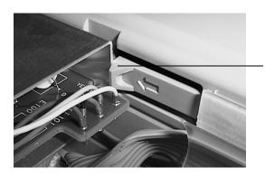
Make sure that shield is locked in place behind this tab
